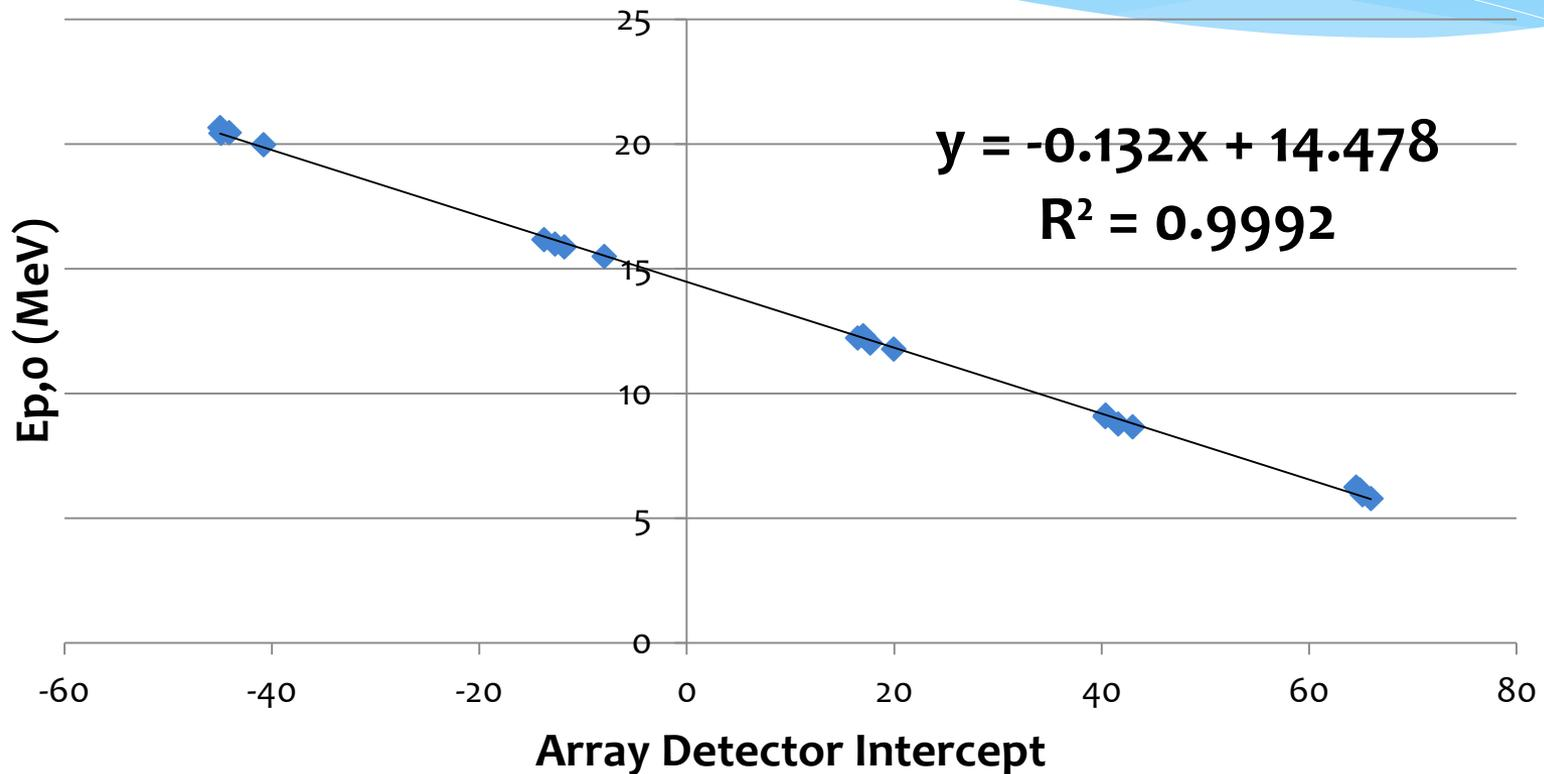
Most Probably Electron Energy at Surface ( $E_{p,o}$ ) vs. Array Detector Intercept
