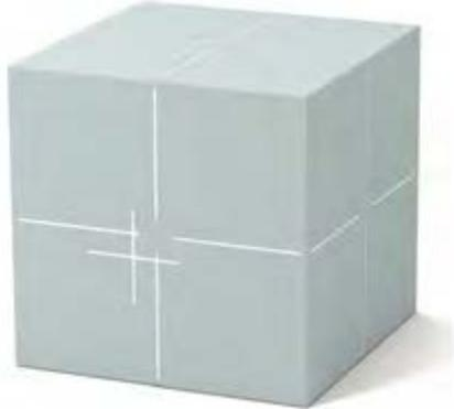
Made from Plastic Water<sup>®</sup> and easy to align, the WL3 phantom is designed for DoseLab's Winston-Lutz analysis. The WL3 phantom contains a hidden 5mm **ceramic** sphere at the center, which is easily revealed during MV and kV imaging. Off-set alignment markers are also incorporated, making the WL3 phantom ideal for checking IGRT coincidence accuracy.
