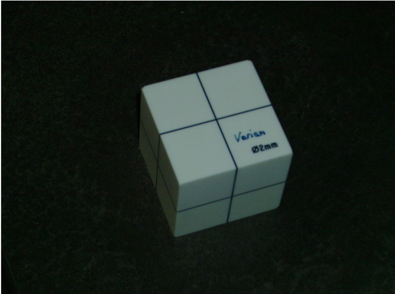
Manufacturer-supplied QA block for CBCT and MV tests
