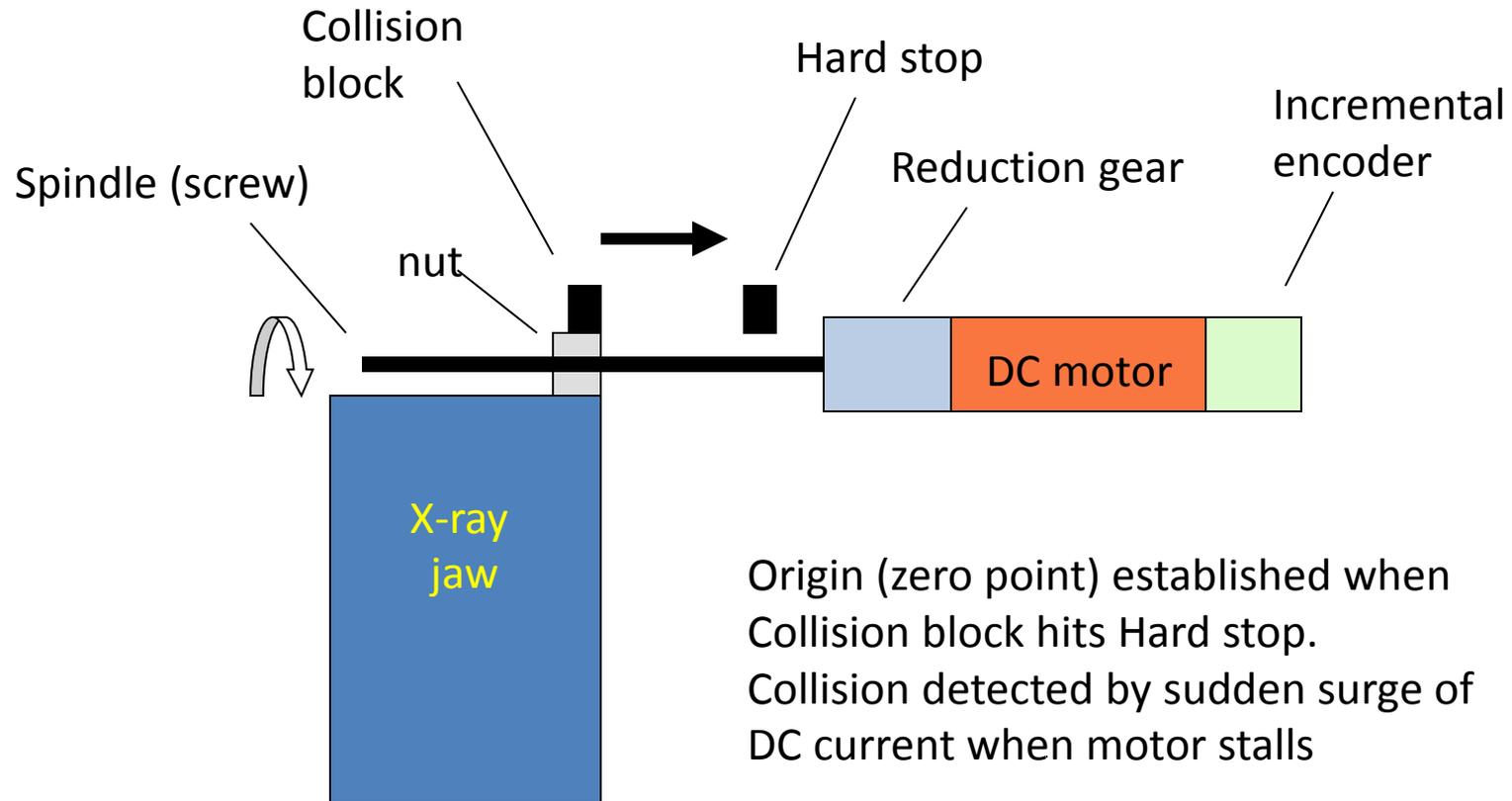
“Software” correction for mechanical imprecision of imaging system. Goal: treatment beam accurately matches images
