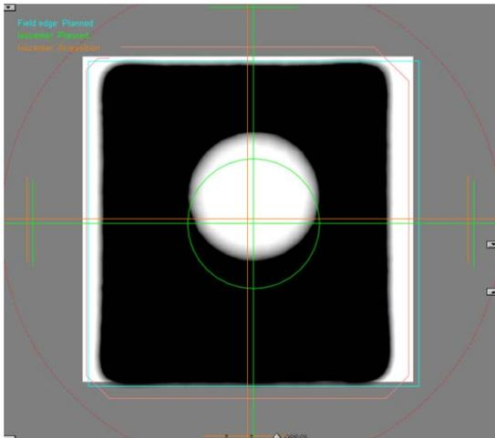
5. Adjust contrast to get sharp outline of lateral field edges. Match edges, record shift distance
