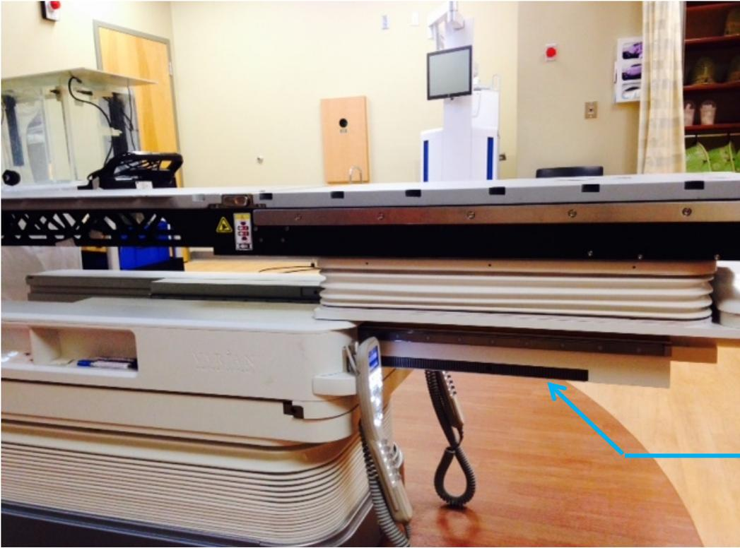
Longitudinal motion control of couch using rack and pinion drive
