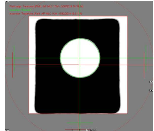
4. Adjust contrast to get sharp outline of sup and inf field edges. Match edges, record shift distance
