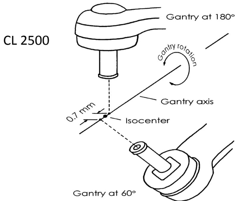
Fig. 2. Due to gantry flex the beam axis shifts as the gantry is rotated.
