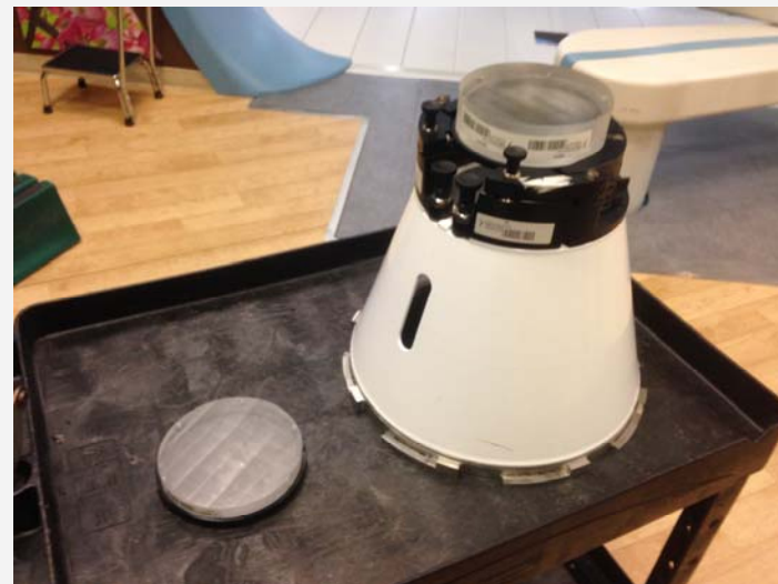
Snout 18cm with 75mm WET range shifter
